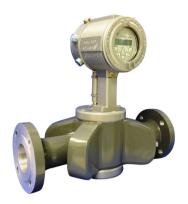
The PanaFlow Z1G gas ultrasonic flowmeter is designed to measure the flow rate of virtually any gas, offering a unique combination of accuracy, range-ability, and reliability in a robust meter design. Employing Ultrasonic time differential technology, the PanaFlow Z1G flowmeter has no moving parts and generates no flow obstruction or energy-robbing pressure drops. Virtually maintenance free, the Z1G will provide years of trouble-free operation with no adjustments, tuning or corrections.
