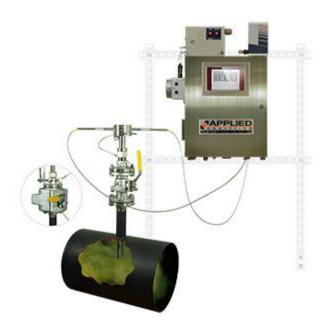
The <u>TLG-837 tail gas analyzer</u> [link to http://aai.solutions/tlg-837-tail-gas-air-demand-analyzer] continuously measures the chemical concentrations of H<sub>2</sub>S, SO<sub>2</sub>, COS, and CS<sub>2</sub> in the Claus process tail gas stream. Using the patented in situ DEMISTER sampling probe and a full-spectrum UV-Vis spectrophotometer, this system provides extremely fast, accurate response for tight process control.
